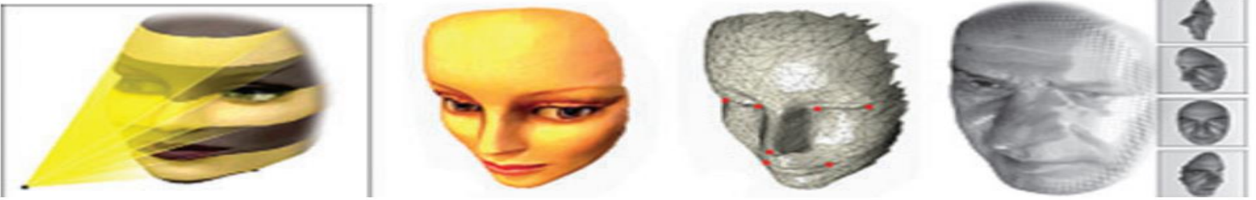
FIG. 2. Structured light and conversion to a triangulated surface or mesh. (Courtesy of Michael and Alex Bronstein.)
